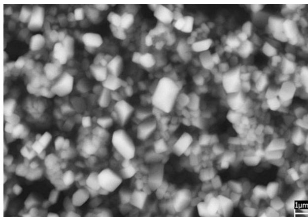
Fig. 4 SEM micrograph of surface of \text{YVO}_4 compound at the end of synthesis at 800 °C during 12 h in air prepared by SGAP
