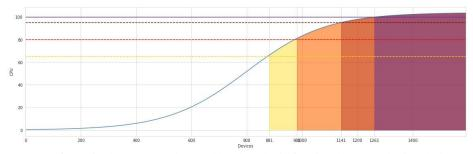
Fig. 2. CPU usage for a single server under workload analysis for simultaneous devices being monitored. (Source: own creation)
