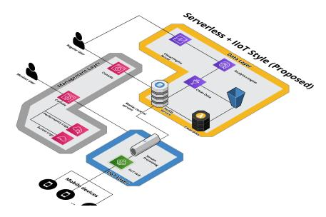
Fig. 4. Serverless architecture proposed using IIoT approach and serverless compo- nents.
