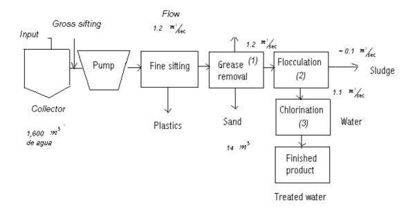
Figure 1. An open and continuous system of sewage treatment
