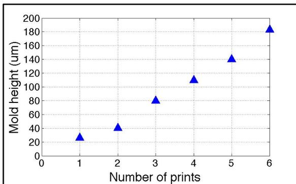
Figure 2: Mold height measurements obtained by feeding through the TPS sheet in the laser printer several times.
