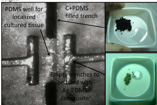
Figure 3: Mixtures of C+PDMS and Ag-PDMS were prepared to be filled into previously defined trenches. Notice how the design defines an area where the tissue culture will be located.
