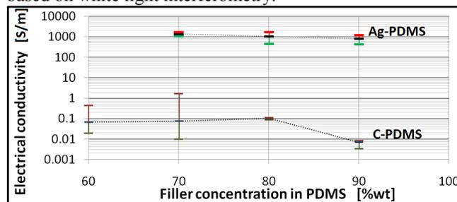
Figure 4: Electrical conductivity of C-PDMS and Ag-PDMS composites as a function of filler concentration and operating voltage. Average values and maximal dispersions are presented over a 0-30V range.
