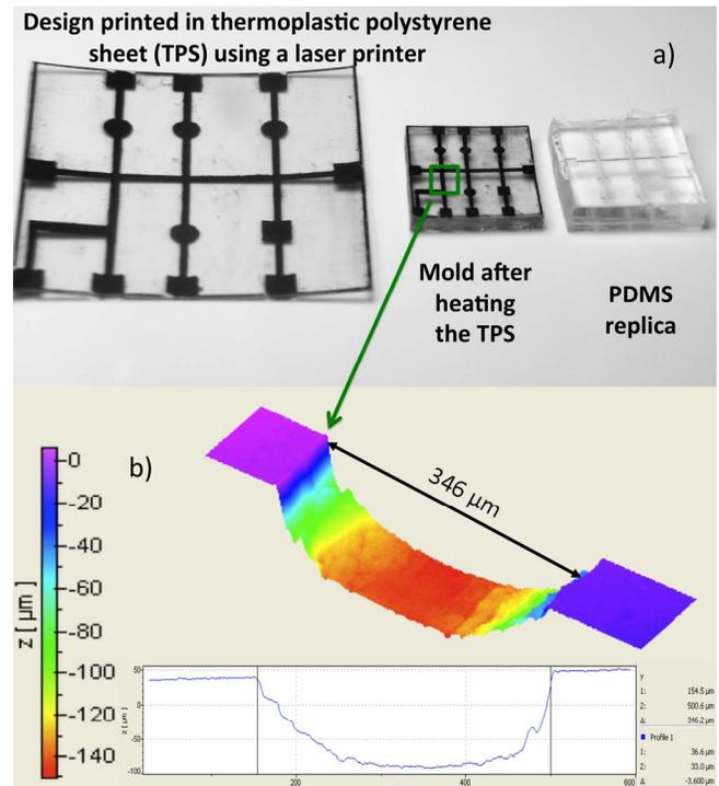
Figure 1:(a) Photograph of the fabrication process showing: printed design on TPS sheet, mold obtained after heating the TPS and its PDMS replica; and in (b) the results of optical profilometer of the trenches cross-section taken by MSA-400 Polytec optical topography system are presented.
