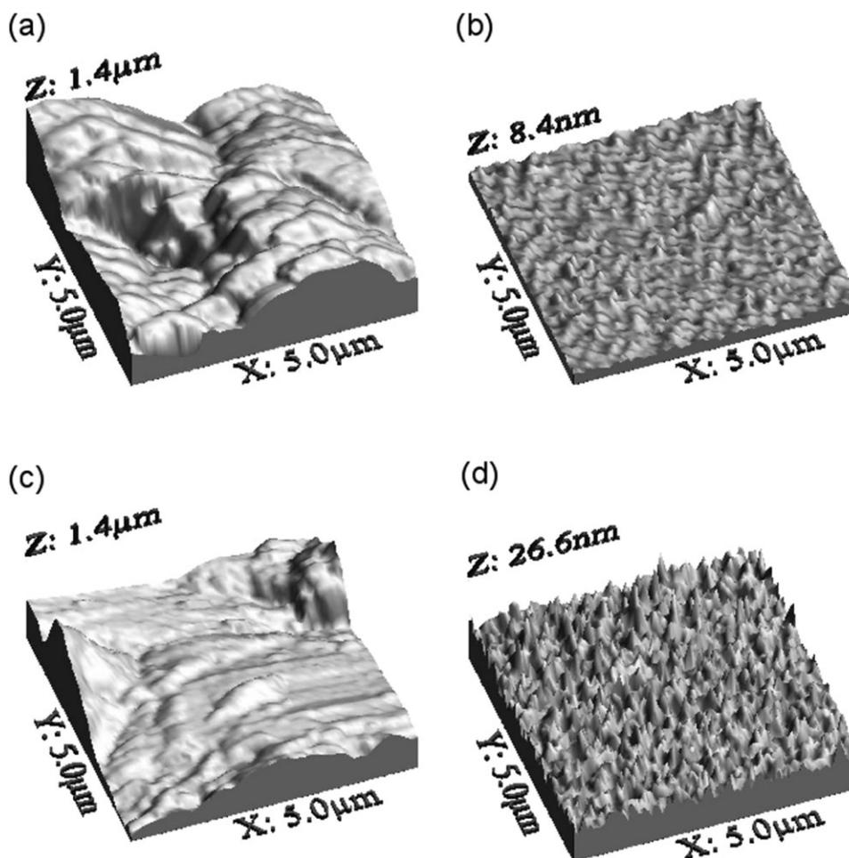
**Figure 1.** AFM images of the test substrates. Vertical scale has been normalized, Z value indicates maximum height in each film. (a) a-C film deposited on the stainless steel sandblasted substrate (a-C r). (b) a-C film deposited on silicon substrate (a-C s). (c) Ti film deposited on the stainless steel sandblasted substrate (Ti r). (d) Ti film deposited on silicon substrate (Ti s).
